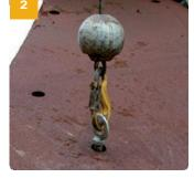
Screw the lifting eye supplied into the centre hole until fully tight. Locate straps or chain through the eye ready for lifting.
