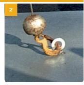
Screw the lifting eye supplied into the centre hole until fully tight (middle 2 holes on the LS range). Locate straps or chain through the eye ready for lifting.
